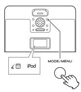
You can also use the FUNCTION button (▲/▼) on the remote control unit to select "iPod".
